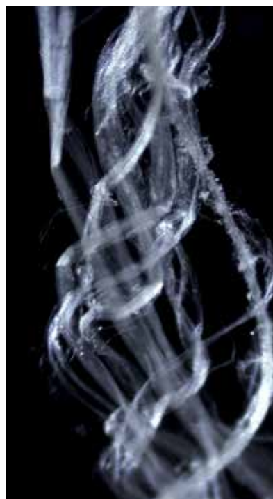
A fibre made from spider silk protein with incorporated antimicrobial peptides.
